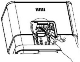
A line drawing showing a hand using a brush to clean the coffee powder outlet. The brush is positioned at the outlet, and the hand is shown in a cleaning motion.            |
