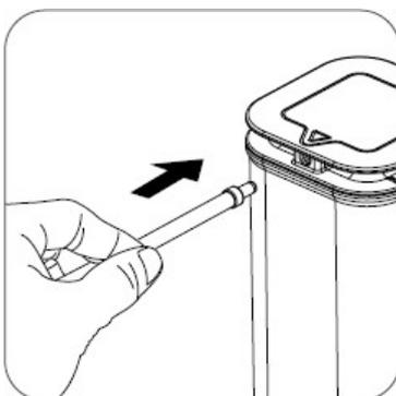
3. Insert the connection milk tube to the rubber outside the lid.
